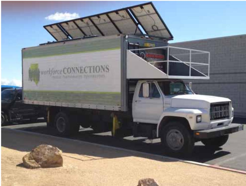
*The Green Mobile Classroom is equipped with STEM interactive labs and hands-on activities. The classroom is powered by solar energy (see photo-voltaic panels on the roof).*
